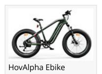
HovAlpha, HovAlpha Step-Through and HovBeta, 26" and 20" fat tire ebikes are perfect for offroad adventures with their extended battery life, incredible speed and stylish design. The 750W hub motor in the rear wheel will provide up to 20 mph (32 km/h) of assist on throttle-only riding or an even faster 28 mph (45 km/h) when the rider uses the highest pedal assist level.
