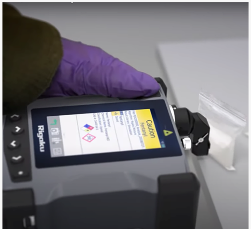
Rigaku ResQ CQL handheld 1064 nm Raman analyzing drug baggie for fentanyl.
