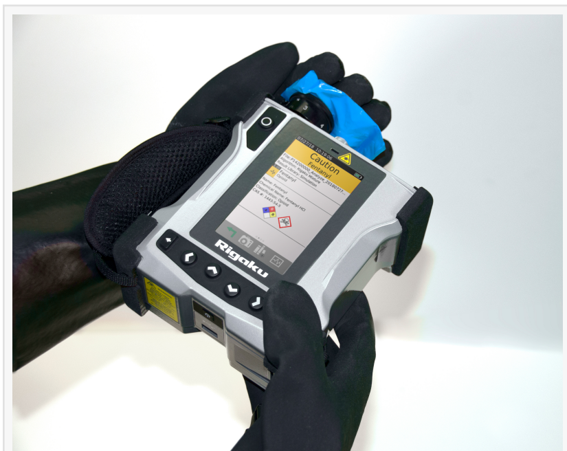
Detecting fentanyl in a drug sample using a Rigaku ResQ CQL handheld 1064 nm Raman analyzer.
