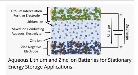
develop their revolutionary Lithium-Zinc Ion (Li-Zn) battery. The Li-Zn chemistry is cobalt and nickel free and utilizes an aqueous electrolyte, which makes this a safe and inexpensive alternative to traditional Lithium-Ion batteries and provides a viable alternative to Lead-Acid and most Lithium-Ion battery applications.
