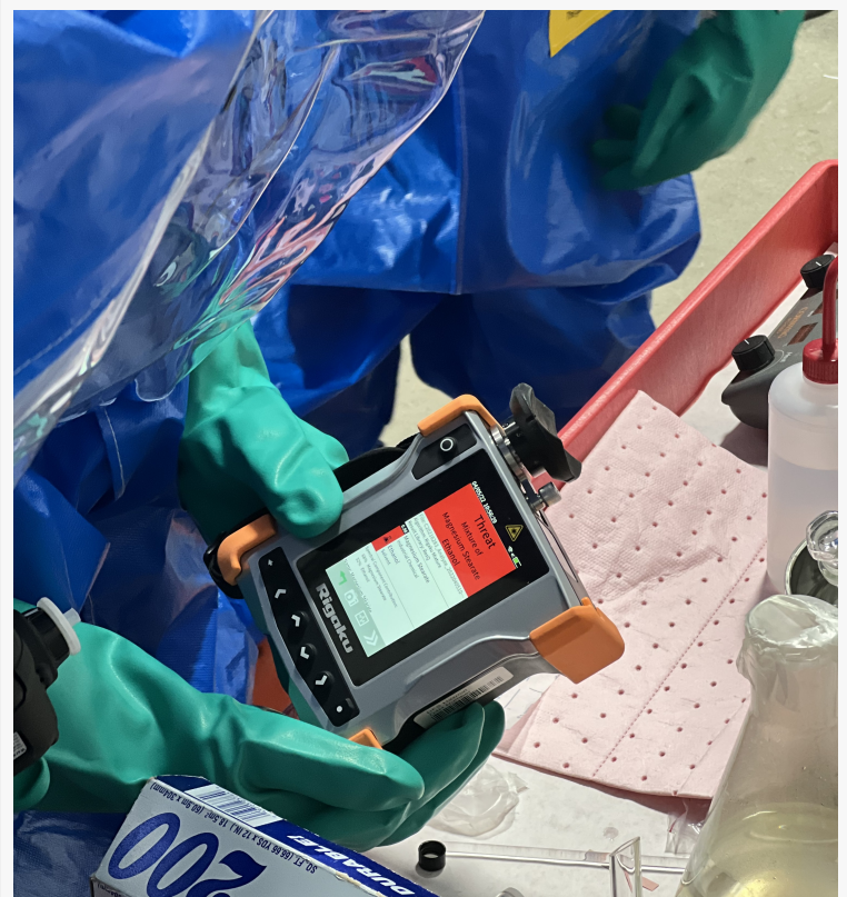
Handheld Raman analyzers from Rigaku used for threat detection by DoD.
