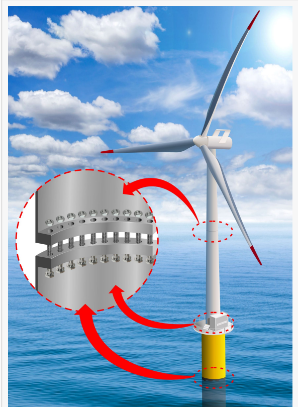
The large flanges on offshore windturbine for tower bases, monopiles and transition pieces need millimeter precision so bolts do not loosen over time.
