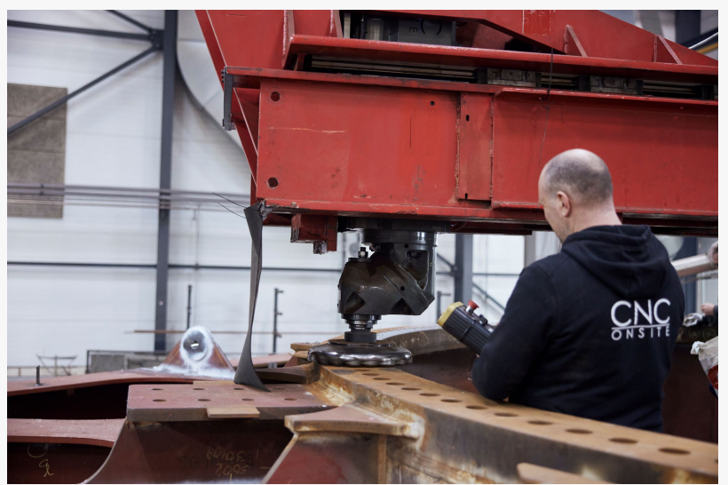
CNC Onsite's Goliath works automatically and delivers millimeter precision for large flanges of up to 10-m diameter
