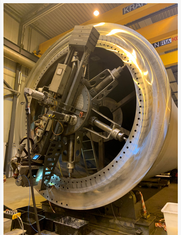
CNC Onsite's new tool works automatically using pre-pogrammed parameters, milling to within two millimeter accuracy
