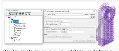
Use Thermal Scaling to quickly deform parts based on temperature changes
