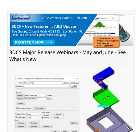
Use Feature Angle Measure to Determine the Expected Angle of Components after Building
