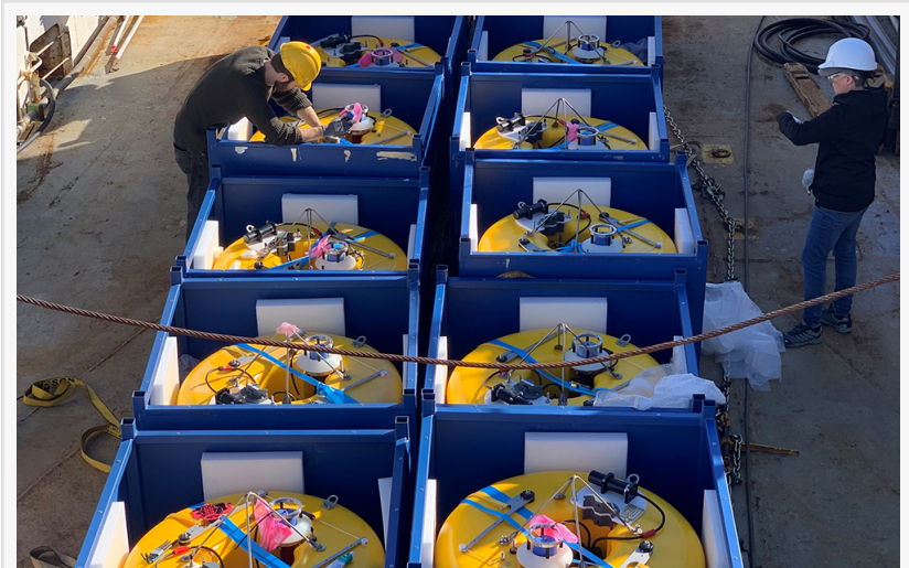
NFSI team prepare Aquarius BBOBS on deck prior to first deployment in November 2021
