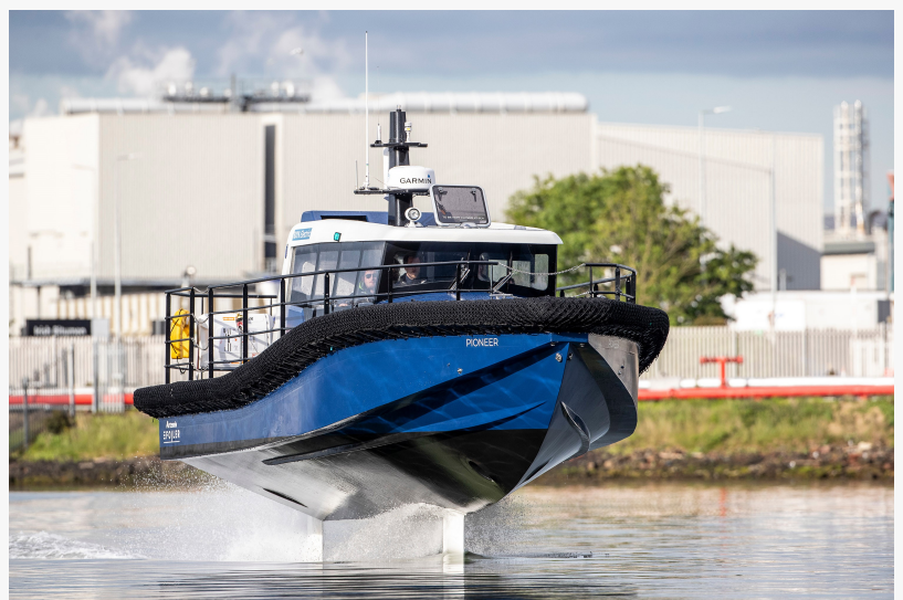
Artemis Technologies' 11.5m multi-purpose, zero-emission workboat foiling in Belfast Harbour
