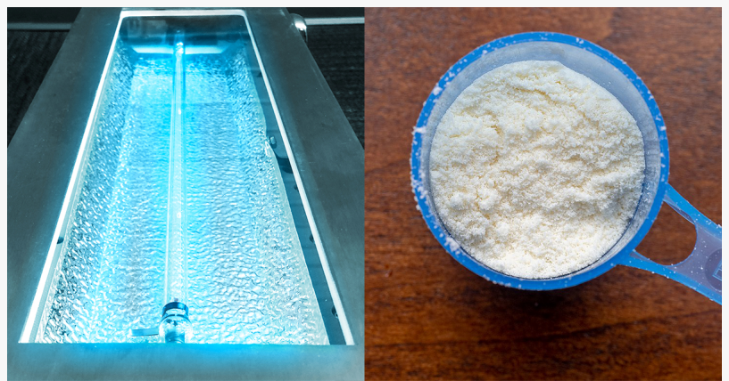
UV-C Lamps can be used to inactivate bacteria in food powders. Baby formula image credit: Ajay Suresh (CC License)
