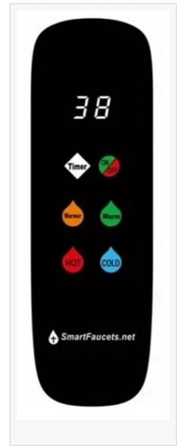
By combining the smart touchpad with the motion sensor faucets, SmartFaucets can now be installed in places with only one sink. This new technology is perfect for a hotel or hospital room. SmartFaucets uses rechargeable hydroelectric powered battery and need only be charged for half hour by hotel/hospital cleaning staff for 2000 uses or one month if used 50 times a day.
