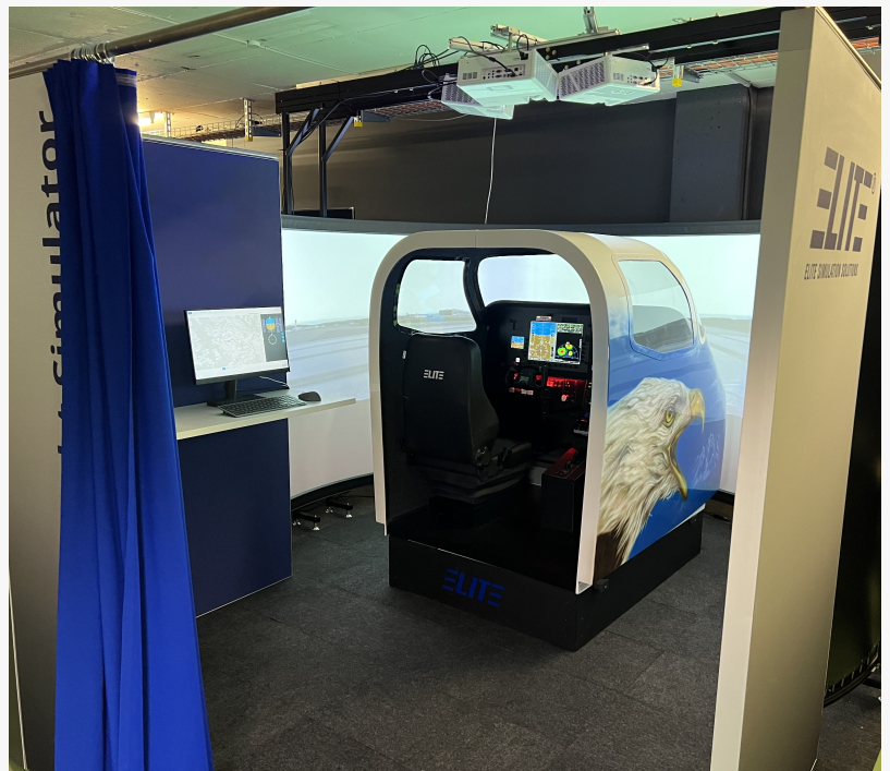
ELITE Evolution S311 FNPT II FSTD with enclosed instructor cabin and curved visual
