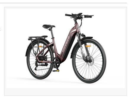
The HovRanger Step-Thru ebike is a simple and effective e-bike for getting around the city and carrying the gear, groceries, or kids. Its upright riding position and suspension fork provide riders with a pleasant riding position. The seat has loads of adjustment and a quick release lever. Hydraulic disc brakes with 180mm rotors stop the bike quickly when engaged. The backlit LCD display is easy to read.
