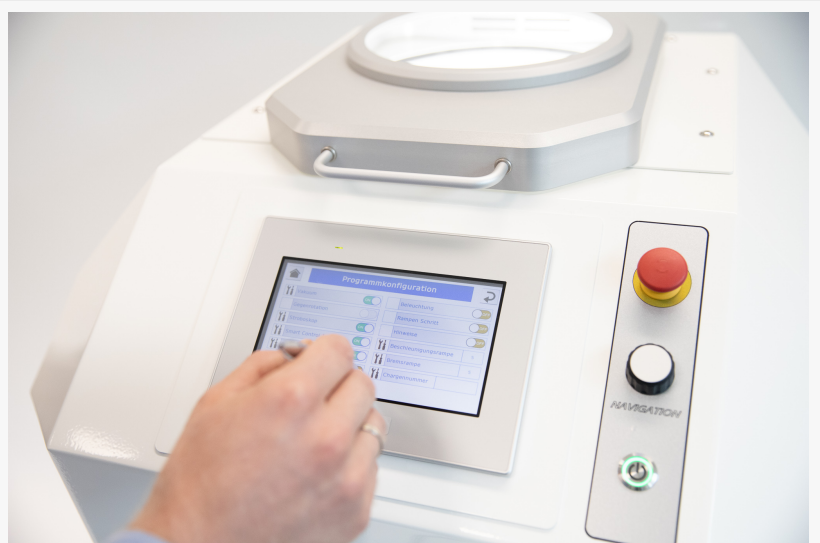
Mixing new formulations for products with the Hauschild SpeedMixer® SMART DAC with sensor integration and automatic pot cooling system
