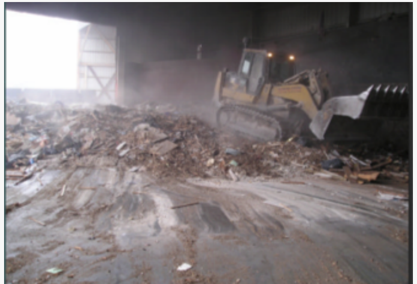
East Coast transfer stations must move fast and furiously and there is little time for waste inspections. They crush the different wastes to maximize the payloads on CSX trains and fleets of long haul trucks. Photo courtesy of the Ohio EPA.
