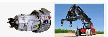
Sigma's EMAX Electric Powertrain for Terminalift's Reach Stacker Vehicles
