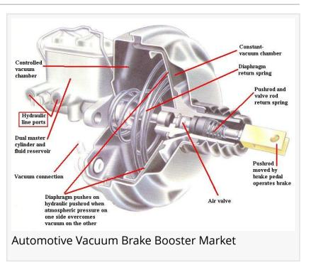
engine compartment under the vehicle's hood, right in the front of the driver's legs. Automotive vacuum brake booster component functions as a force multiplier. Automotive vacuum brake booster utilizes engine vacuum in order to multiply the unbalanced force exerted by the car driver upon the braking pedal before sending it further to the braking master cylinder.
