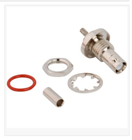
IP67 HD□BNC connectors utilize the trusted bayonet□style positive locking mechanism for easy installation and secure mating. This interface is available in a number of both 50 and 75 ohm configurations including straight and right-angle versions for cable mount applications, and features a closed entry interface. HD□BNC connectors are a popular choice for broadcast, military and industrial applications equipment.
