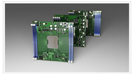
congatec extends its Intel Xeon D-2700 processor based Server-on-Module portfolio by launching 5 new modules in the compact COM-HPC Server Size D class
