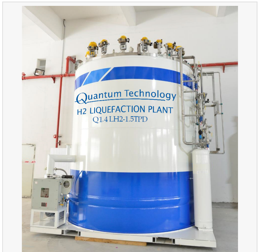
Hydrogen liquefier 1.5 ton per day in Squamish, BC
