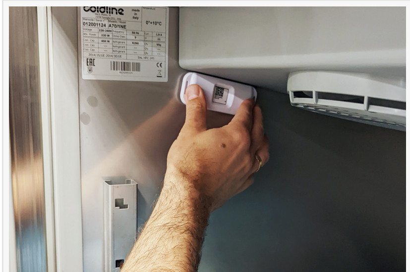
Sensor installation in freezer with range extender
