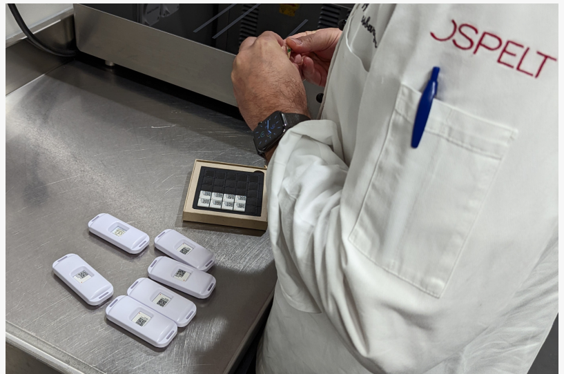
Peel and stick the sensors into the range extenders
