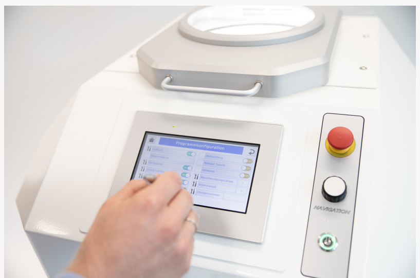
Mixing new formulations for products with the Hauschild SpeedMixer® with sensor integration and automatic pot cooling system
