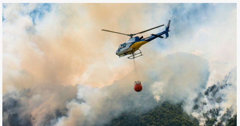
Bambi bucket system used by Aragón's aerial firefighting fleets
