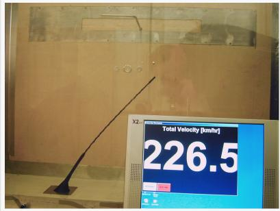
Car antenna undergoing testing in Airflow Sciences' in-house wind tunnel.
