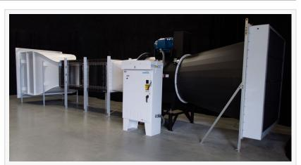
This custom wind tunnel was recently designed and manufactured by Airflow Sciences. It includes all the standard wind tunnel features plus the ability to introduce water droplets to test vehicle components in various rain conditions.
