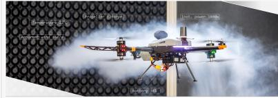
WindShape can recreate any kind of flight condition in a controlled environment
