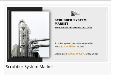
A scrubber system is a system that is used to remove harmful materials from industrial exhaust gases before they are released into the environment. These systems use a slurry or dry reagent that is injected into a polluted exhaust stream to eliminate acidic gases. Scrubber systems can perform flue-gas condensation for heat recovery.
