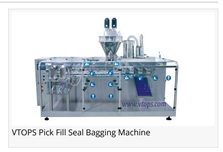
Designed specifically to fit the existing bag sizes of its client that packages ground coffee, Zhengzhou Vtops Machinery Co Ltd says that the automated system conveys ground coffee from a hopper conveyor to an auger dosing system via a screw conveyor.
