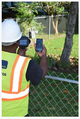
quantitative, mid-infrared Optical Gas Imagers (OGI) that are utilized to comply with natural gas
