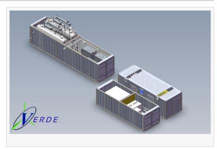
to the popularization of "green hydrogen". The system features advanced water electrolysis hydrogen production patented technology with a total footprint of only 2 of 30ft containers and 1 of 40ft container. It can be modularized to 20MW, 500MW, or larger module scales. With a 1000Nm3/h (2000kg/day) hydrogen capacity, purity can reach 99.999% after purification, and the maximum output pressure is 3MPa.
