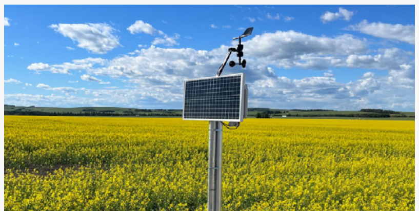
Qube device monitoring for methane emissions at an Arc Resources gas site.
