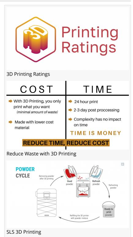
Similar problems occur with various frequently used metal powders, where the SLS process's byproducts might compromise the chemical integrity of any powder left behind. Additionally, even with the highest degree of accuracy during the sintering process, excess particles in the powder bed will unavoidably fuse without adhering to the part, altering the material's size distribution and resulting in inconsistencies if reused.
