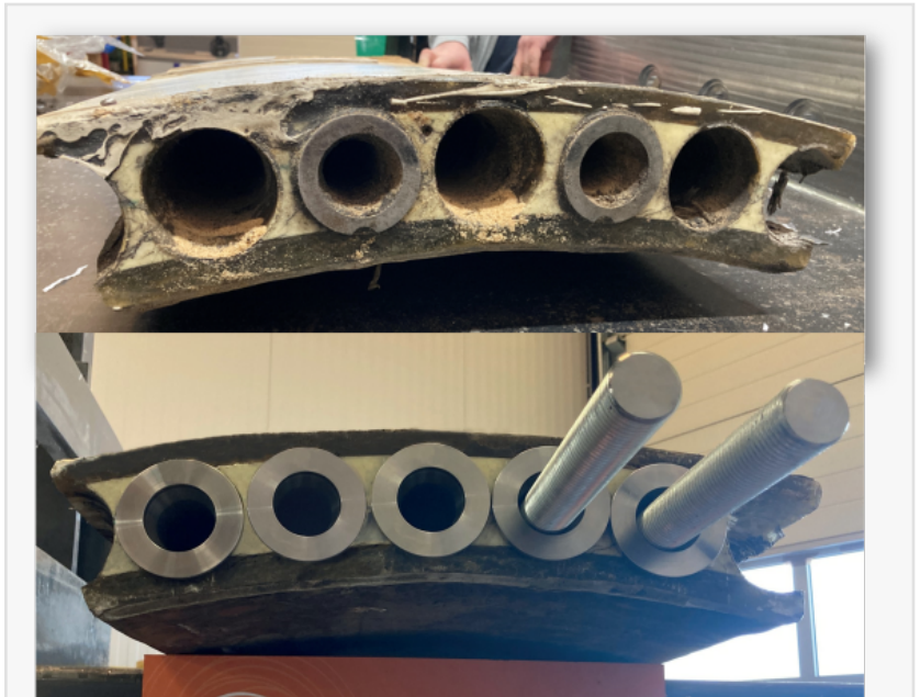
Before and After: Damage to blade root inserts (above) and after
