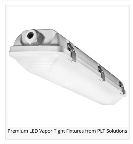
durable polycarbonate with a gray finish and solid steel latches. The tapered ribbed lens and LEDs are built into the fixtures with a single integrated piece. IP65 rated, these fixtures are built to restrict the entry of dust and protect them from being damaged when exposed to harsh weather or washed with high pressure blasts of water.
