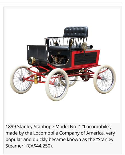
1 "Locomobile", made by the Locomobile Company of America, was the auction's top lot, selling for \$44,250. It was very popular and quickly became known as the "Stanley Steamer" due to its quiet but powerful two-cylinder steam engine. The literature boasted it "weighs less than 400 pounds and is odorless and noiseless when in use."
