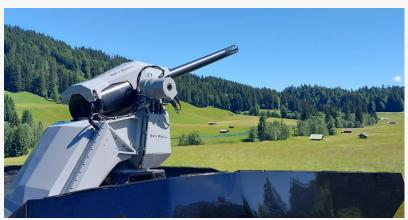
SkyWall Auto can be used as a standalone drone capture system but can be integrated with a drone detection and security system to offer a highly capable and easy-to-operate counter-drone solution.
