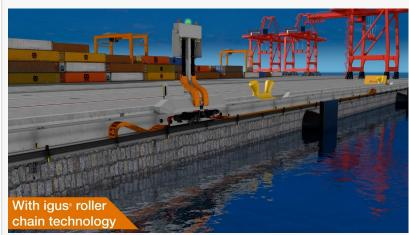
The readychain® iMSPO (igus Mobile Shore Power Outlet) is a self-propelled socket for shore power connection of container ships. (Source: igus GmbH)
