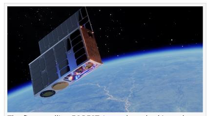
The first satellite, FOREST-1, was launched in early 2022 with a plan to build up a constellation of 100 nanosatellites by 2026. The satellites are equipped with novel thermal-infrared cameras that speed up wildfire detection and monitoring notifications
