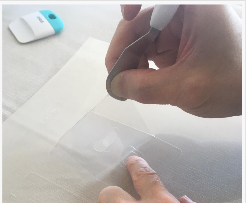
Once cut by the cutting machine, the material can easily be peeled away from the backing
