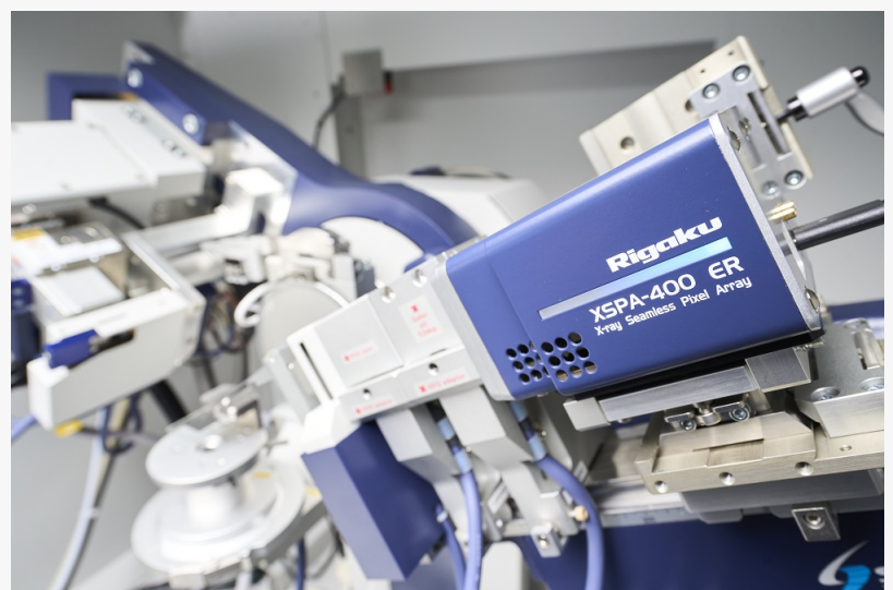
The new Rigaku XSPA-400 ER XRD detector integrated into a SmartLab diffractometer.
