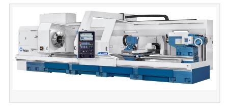
for machining large parts. It is built with a Romi-made monoblock cast iron bed that absorbs machining efforts and vibration, making it highly rigid, stable, and accurate.
