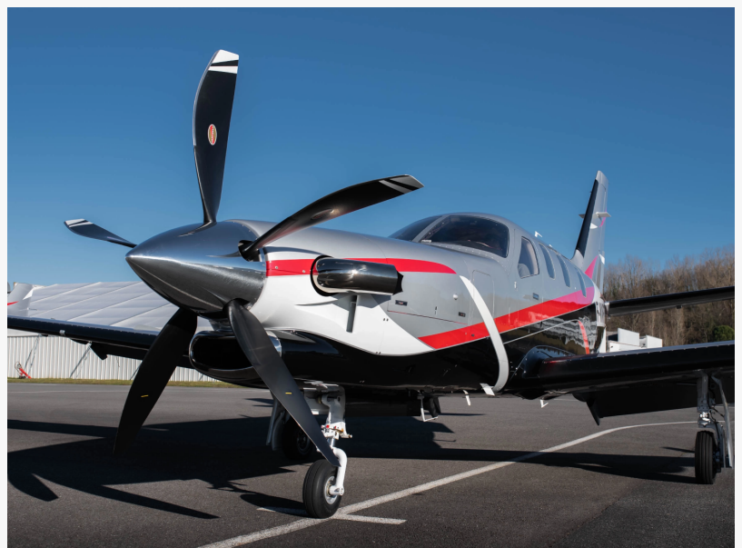
The lightweight Raptor five-blade composite propeller from Hartzell has been specifically designed to reduce overall weight and improve the TBM 960's takeoff distance, climb and cruise speeds.
