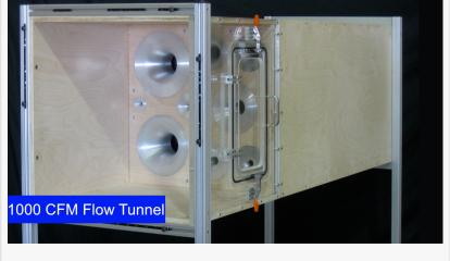
engineers that plan to install these products need to know their impact on the whole system, be it a large ventilation system or a small air purifier system. Often a fan or HVAC vent is sent to a flow analysis lab for such testing, but this is only financially reasonable if such testing is rarely
