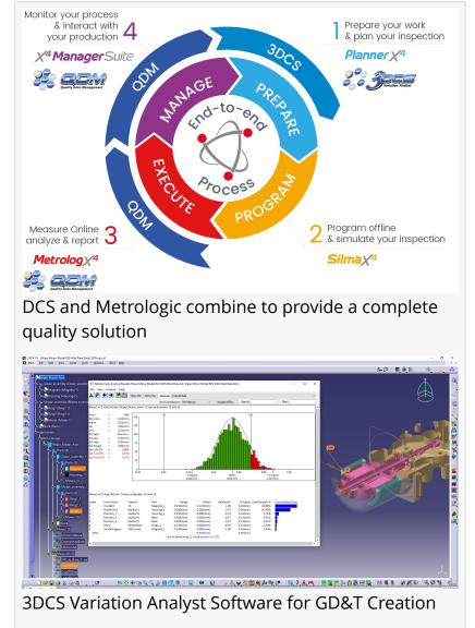
During the digital design phase, 3DCS, a variation analyst tool integrated into CAD, provides the tools to test, simulate, and create robust designs. The output from these models is a set of optimized GD&T, that is, set up to reduce manufacturing costs in noncritical areas, and honed for areas found critical to quality and at risk of non-conformance. This output GD&T is the driving force of the process, associated to CAD and machine readable for consumption downstream.
