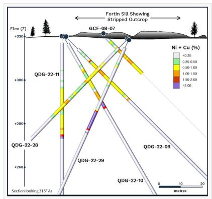
Drill section showing the locations of selected holes completed at the Fortin Sill Ni-Cu-PGE Zone in relation to historical hole GCF-08-07 and the Fortin Sill Zone discovery outcrop.
