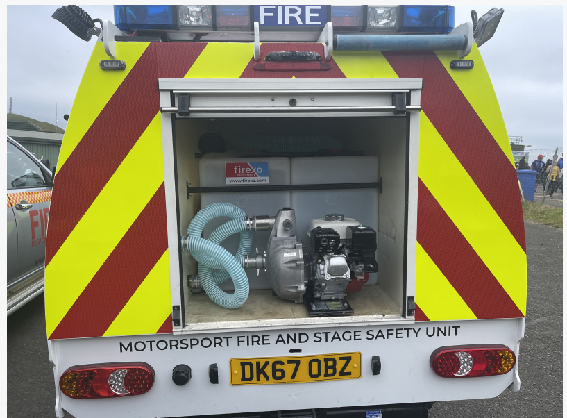
Firexo Liquid Pump at The Rear of Our Knockhill Emergency Response Vehicle
