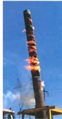
Figure 1 – Untreated Wood Pole Burning
