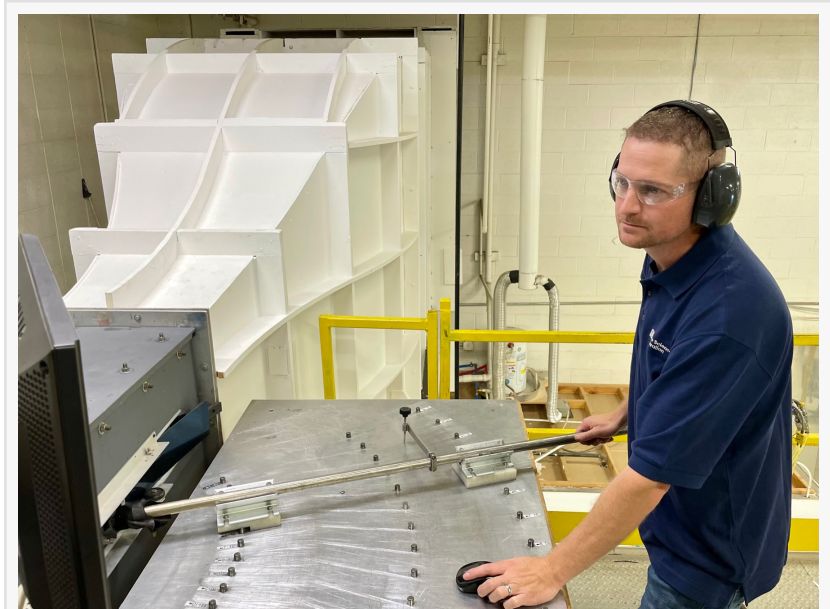
Probe calibration in progress using the wind tunnel at Airflow Sciences' flow lab in Livonia, MI.
