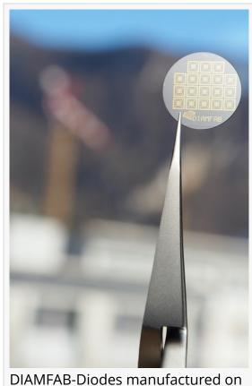
DIAMFAB-Diodes manufactured on a diamond substratre
