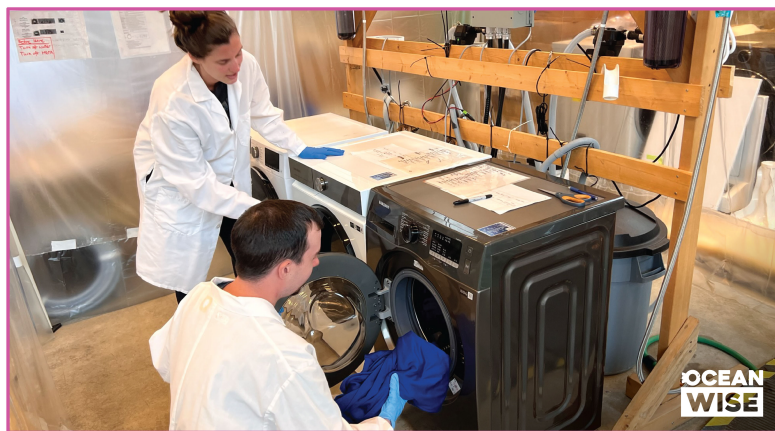
Ocean Wise Plastics Lab researchers conducting wash cycle testing
