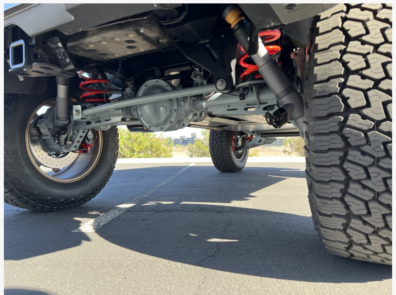
W463A IFS G-Wagen portal conversion demonstrating clearance.
