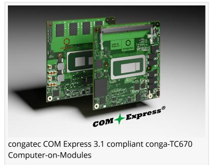
speed interfaces such as PCIe 4.0 and USB 3.2. As upgrades of the already existing family of COM Express Type 6 modules, the new 3.1 compliant modules offer up to 14 cores/20 threads. With these new modules, customers can now give their designs a performance boost that is compliant to this officially ratified specification. This delivers maximum design security and safeguards reliable high-performance roadmaps for existing COM Express designs long into the future.
